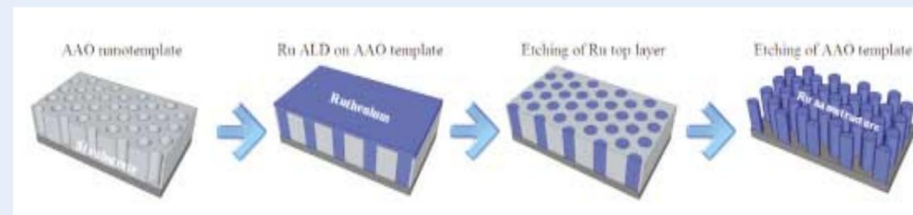
Schematic drawings of process flows for Ru nanodot or nanowire arrays on Si substrate.
