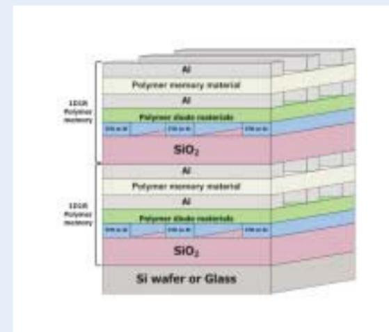
Fig. 2. A schematic structural diagram of the 3D array nonvolatile WORM memory devices.
