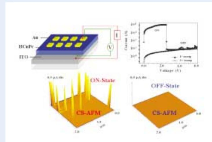
Fig. 1. A schematic structural diagram of the nonvolatile WORM memory device based on HCuPc polymer thin film. A typical current-voltage curve of the ITO/HCuPc/Au devices. Current sensing atomic force microscopy (CS-AFM) images of HCuPc polymer films coated onto ITO and Au substrates.
