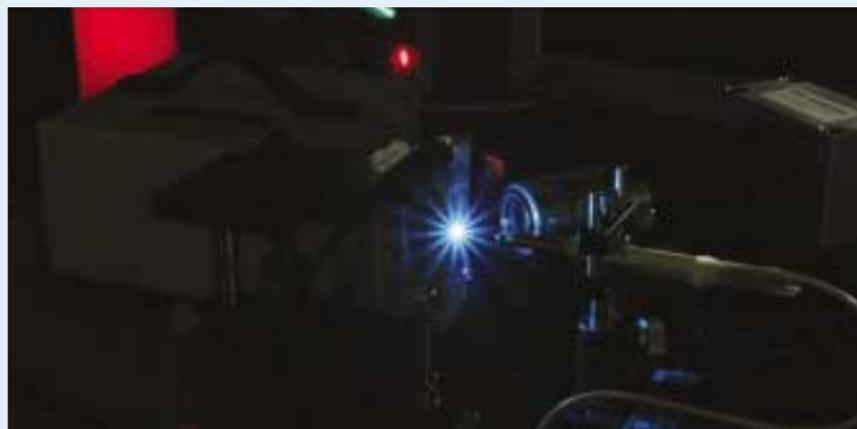
A blue photonic-quantum-ring laser showcases 3D whispering-cave-mode emission with ultra-low-threshold current less than that of VCSELs or LEDs.
