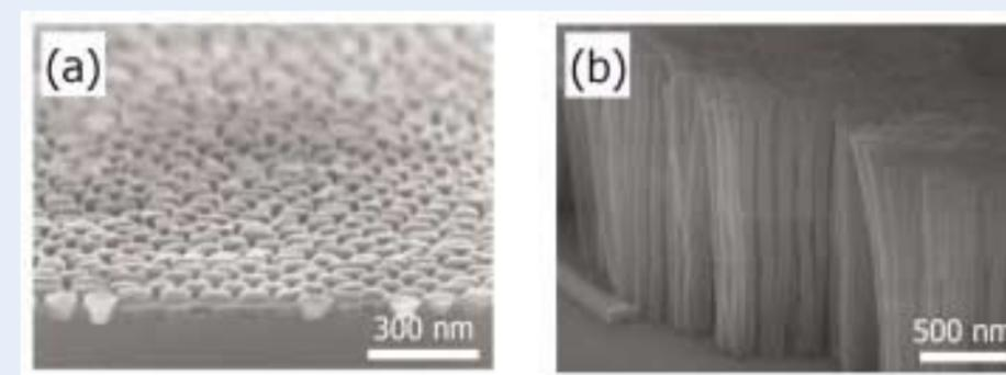
FE-SEM images of Ru nanostructures on Si substrates: (a) the tilt view image of Ru nanodot arrays on Si substrate, (b) the tilt view image of Ru nanowire arrays on Si substrate.
